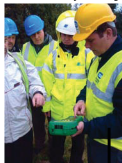
Measurement of earthing resistivity.
